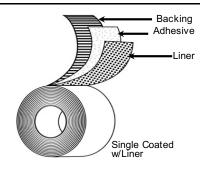
**Backing:** Exterior-Grade Aliphatic Polyurethane
