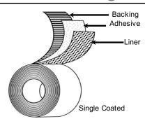
**Backing:** Exterior-Grade Aliphatic Polyurethane
