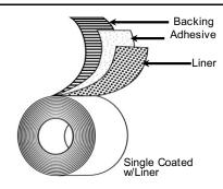
**Backing:** Interior-Grade Aromatic Polyurethane
