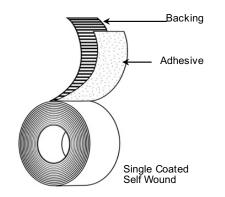
Backing:Embossed PolypropyleneAdhesive:Rubber (RF409)Liner:N/AColors:Clear, Tinted Red
