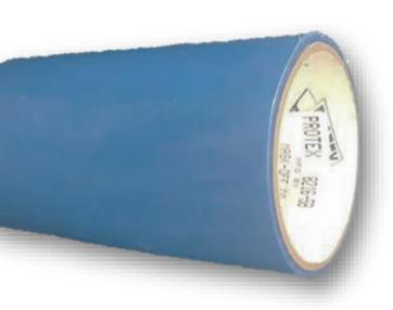
PROTEX 8216-5B is a 5 mil polyester film with an acrylic latex adhesive, tinted blue, designed to protect various metal surfaces including polished, clad, bare and heat treated aluminum, stainless steel and various coated and un-coated plastic surfaces, e.g. stretched acrylic, Plex II, cast acrylic, and polycarbonates. PROTEX 8216-5B is capable of withstanding temperatures up to 325 degrees and prolonged outdoor exposure. Chemical resistance recommended only after thorough initial testing.
