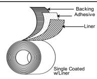
**Backing:** Exterior-Grade Aliphatic Polyurethane
